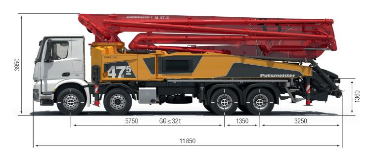
Note: Standard version. Dimensions and weights depend on truck, pump model and equipment. Dimensions in mm, MB-Arocs 4143 as example.
